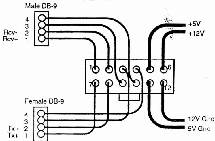
This diagram illustrates the DB9 connectors and the power supply connections to the intercom master box. The large connector illustrated here is actually contained within the master box assembly.
