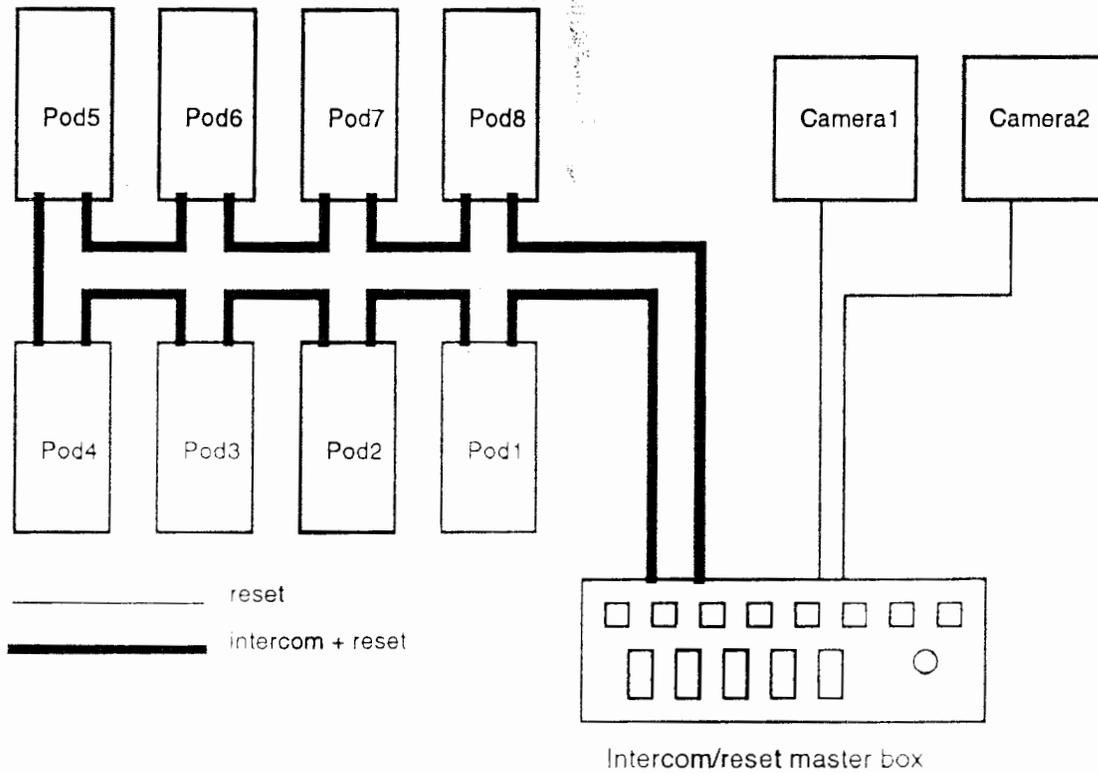
The network chain is terminated at the top of each cockpit. One network line comes into the cockpit from the previous cockpit, and one goes out of the cockpit to the next one. The line going into the cockpit should be terminated with a free hanging female DB9 connector. Likewise, the network line exiting the cockpit should be terminated with a free hanging male DB9 connector. This is represented by diagram #3.
